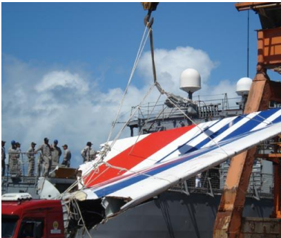
Fig.89 A fragment of the vertical tail stabilizers of the Airbus A330-203 on flight 447, found and raised from the seabed by a Brazilian Navy frigate Photo by: Roberto Maltchik Repórter da TV Brasil
