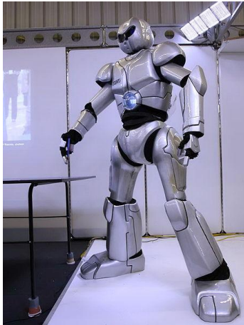
Fig.57 TOSY 2: an android robot with artificial intelligence for playing table tennis.
